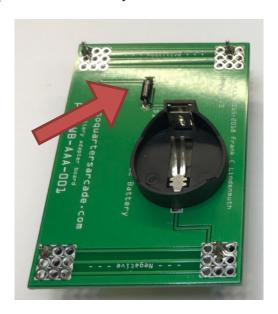
The arrow in the pic of the WPC logic board points to positive end.
