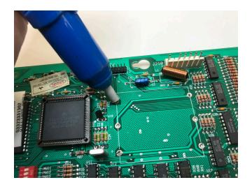
Remove the battery from the CR2032 battery holder before installing it on your logic board. Make sure you observe the polarity markings on both the battery board and your game's logic board. Match the positive-to-positive and negative-to-negative. As a side note, the diode on the battery board points towards the positive side so you can also point diode end to the positive side of the logic board. Arrow in pic below denotes diode and positive end of battery board.
